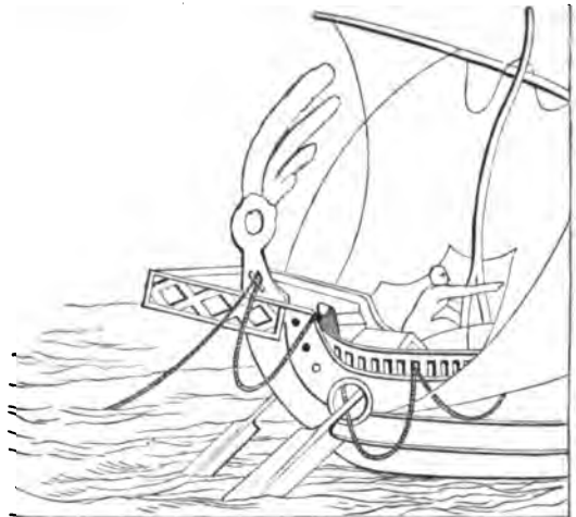
Stern of an Ancient Ship, showing the "Rudders." (From a painting in Herculaneum representing the desertion of Ariadne.)
